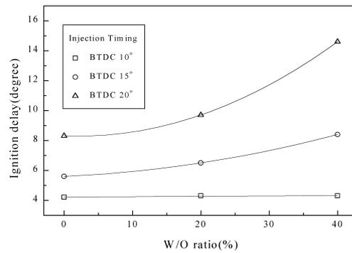
**Figure 8** Ignition delay with respect to the W/O ratio
