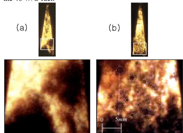
**Figure 9** Magnified images for the (a) diesel and (b) 20 W/O fuel both with the injection timing of BTDC 10
