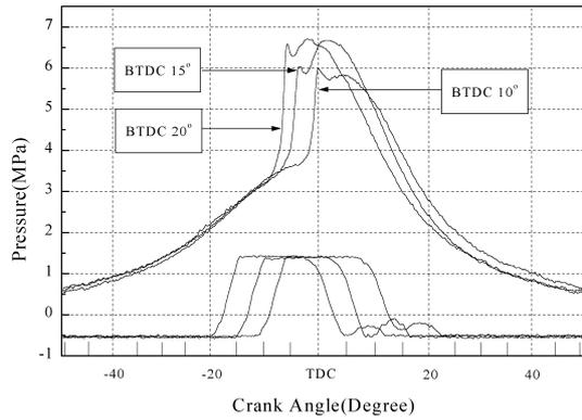
**Figure 3 Pressure and needle lift data for the diesel fuel(0 W/O) with the injection timings of BTDC 10, BTDC 15 and BTDC 20**
