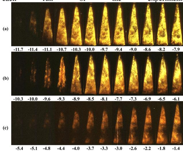
**Figure 7** Flame images for (a) the diesel fuel with the injection timings of BTDC 20, (b) the 20 W/O fuel with the injection timings of BTDC 20, (c) the 40 W/O fuel with the injection timings of BTDC 20 (The negative numbers below images represent the crank angle)
