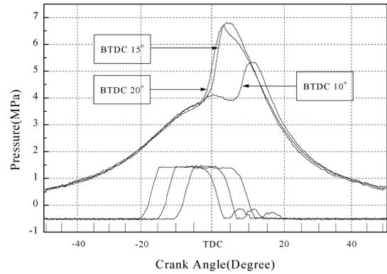
**Figure 5 Pressure and needle lift data for the diesel fuel(40 W/O) with the injection timings of BTDC 10, BTDC 15 and BTDC 20**
