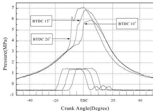
**Figure 4 Pressure and needle lift data for the diesel fuel(20 W/O) with the injection timings of BTDC 10, BTDC 15 and BTDC 20**
