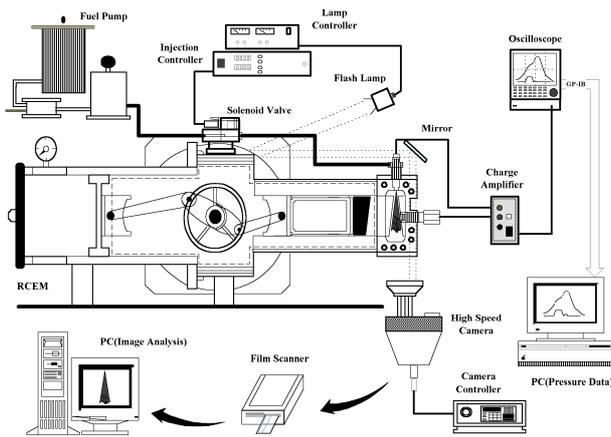
**Figure 1 Schematic diagram of the RCEM**
