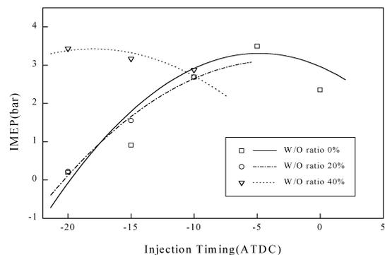
**Figure 6 IMEP of the 0, 20 and 40 W/O fuels with respect to the injection timing**
