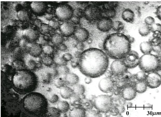
**Figure 2 Microscopic photograph of the 40 W/O fuel with 0.1% stabilizing agent**
